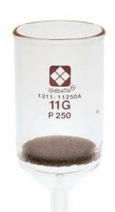
EXTRA COARSE [160-250pm] [liquid and gas dispersion, coarse filtration]; COARSE [40-100pm] [preparative fine filtration and work with crystalline products, mercury filtration]; PARTLY COARSE [16-40pm] [analytical work with medium-fine precipitates, fine gas filtration]; MEDIUM [10-16pm] [analytical fine filtration preparation work with the finest precipitates]; FINE [4-5.5pm] [filtration of fine precipitates, mercury valve, extraction apparatus.]
